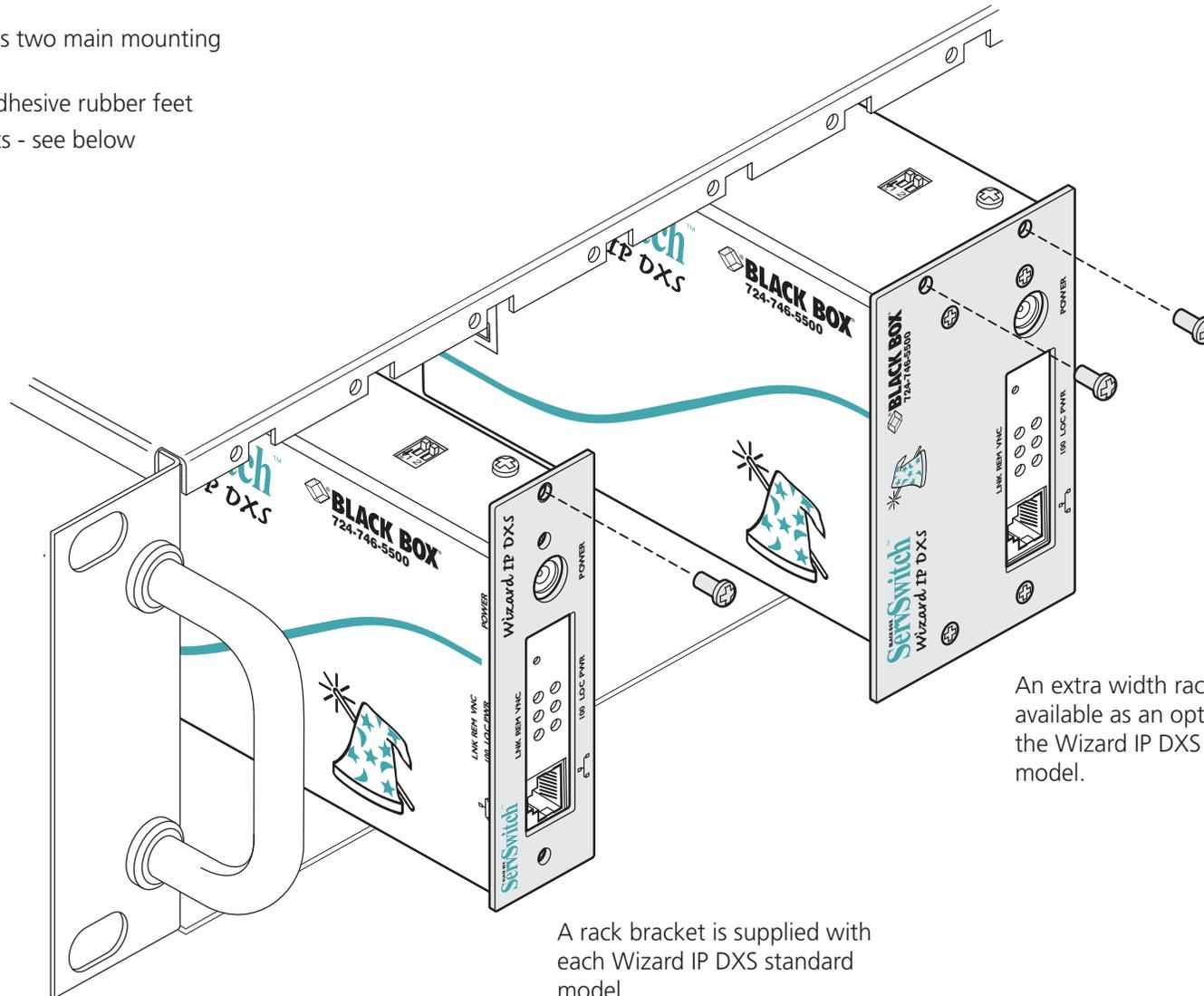
A rack bracket is supplied with each Wizard IP DXS standard model.
