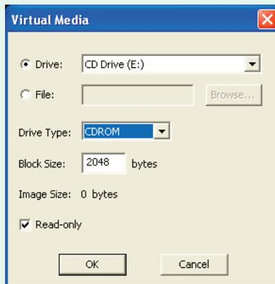
Select the required storage device or file/folder, choose an appropriate 'Drive Type' (virtual CD, floppy or disk (directory)) and click OK. The selected device will be tagged for transfer but no other action will take place at this point.
