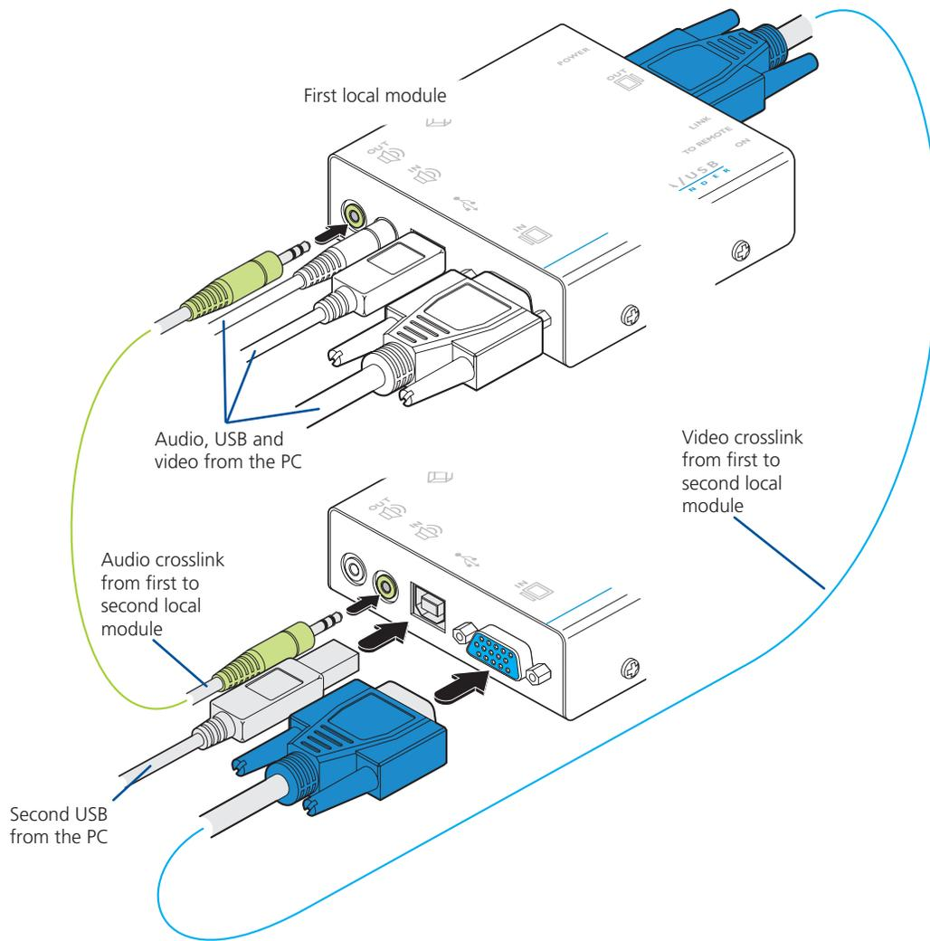
Figure 3-23. Interconnections required for a dual user configuration
