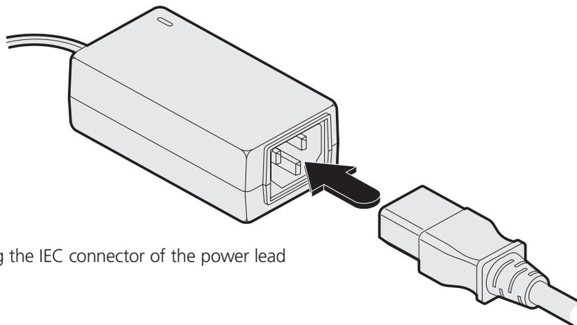
Figure 3-13. Inserting the IEC connector of the power lead
