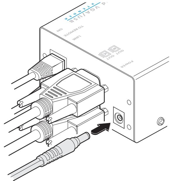
Figure 3-12. The use of a power supply on single-variant local modules is optional. Dual-variant local modules always require a power supply.
