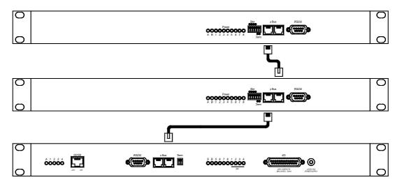
2. Allocate an address to each Satellite by positioning the address selection DIP-switches marked "Slct" on the front panel according to the following table.
